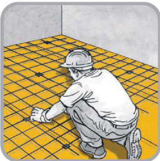
Placing reinforcement mesh
