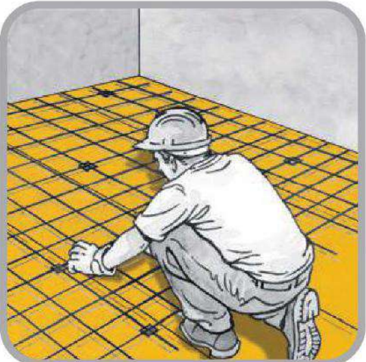
Placing reinforcement mesh
