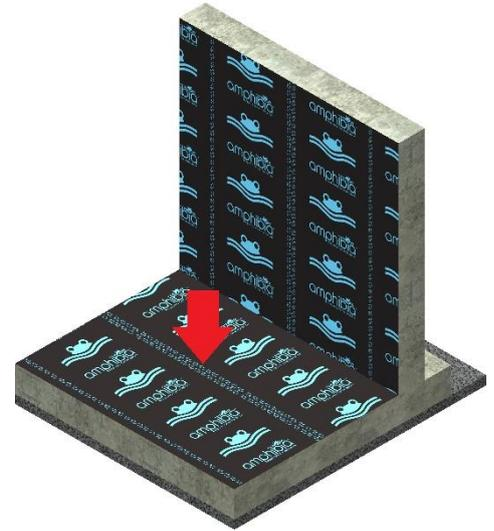
4. **AKTI-VO 201**, must be placed at the bottom of the vertical wall on the existing foundation slab (before casting the new structure) between the Amphibia membrane and the concrete wall. For a proper use of the tool, must be used the button " WALL: SWEEP", and select the walls on which you want to paste the component after choosing it correctly from the REVIT device.
