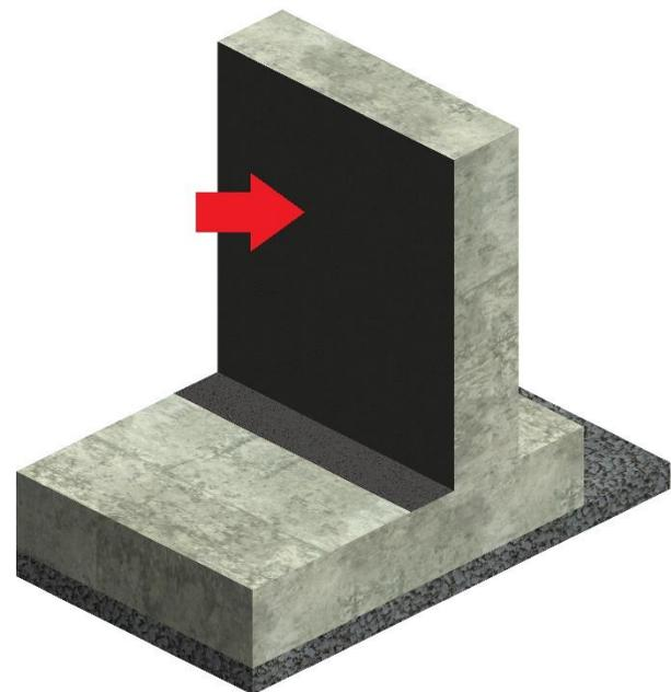
10. **PLASTIVO 250, HORIZONTAL EDGE**, must be installed at the bottom of the vertical walls on the existing foundation or lean concrete, (before casting the new structure) for a width equal to approx. 20cm. For a proper use of the tool, use the button "WALL: SWEEP", and select the walls on which you want to paste the component after choosing it correctly from the REVIT device.
