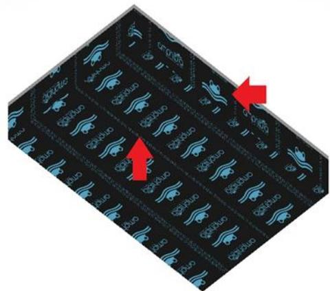
5. **WT102** or **WT CONSTRUCTION** is a hydro-expansive joint, it must be applied on the middle of construction joints between the foundation and vertical wall and it must guarantee a minimum cover of 8 cm per side; For a proper functional response of the panel commands, the button "WALL: SWEEP", and select the walls on which to paste the component after choosing it correctly from the REVIT device.
