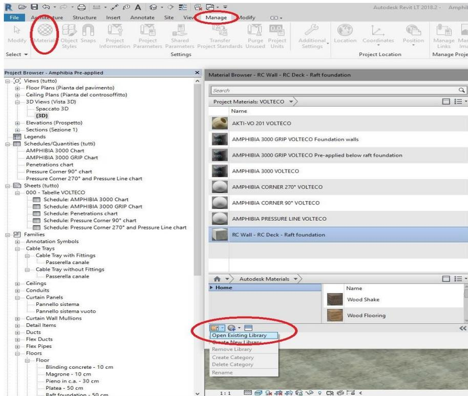
2. **Load "VOLTECO amphibia" texture** to define the appearance of Amphibia 3000 and Amphibia 3000 Grip technologies.
