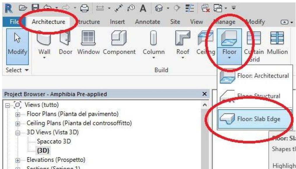
5. **AQUASCUD H.10 LINE** must be installed all along the edges of the terrace. Use the "FLOOR – SLAB EDGE" and pick on the edge to apply the element.
