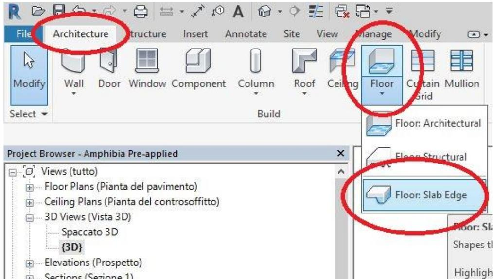
4. **GARVO 3 e 5** must be installed on the fractionation and/or structural joints. Use the "FLOOR – SLAB EDGE" and pick on the edge to apply the element.
