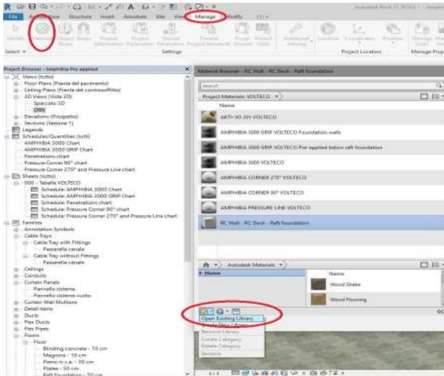
2. **CONNETTORE 20 and BI FIX**, the CONNETTORE 20 must be installed on the wooden beams; For a proper functional response of the panel commands, use the button "COMPONENT", and select the position on which you want to paste the component after choosing it correctly from the REVIT device. In the end, in the abacus, "CONNETTORE 20 and BI FIX", to simplify the automatic calculation, manually insert the number of connectors in the column "N° connectors tot".
