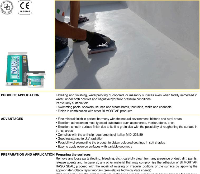
High-pressure clean the surface until it is soaked and remove excess water before applying the product. Seal any localised water flows with TAP 3/I-PLUG rapid-setting hydraulic mortar (see relevant technical data sheets).
